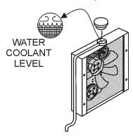
Figure 18. Radiator Coolant
